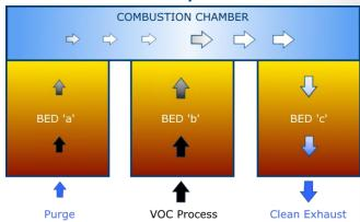
The 3- bed RTO is similar to the 2-bed RTO. The VOC laden air stream enters the first heat exchange bed where the stream passes directly through the media where it is preheated en route to the combustion chamber where a burner adds any heat necessary to reach optimum combustion temperature and complete the oxidization process.
