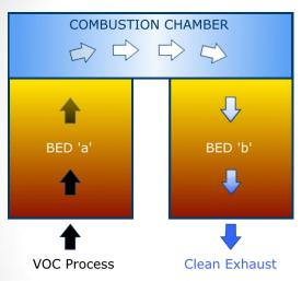
The VOC laden air stream enters the first heat exchange bed where the stream passes directly through the media where it is pre-heated en route to the combustion chamber where a burner adds any heat necessary to reach optimum combustion temperature and complete the oxidization process.
