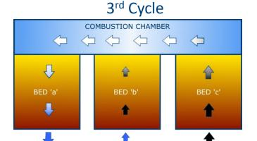
The bed which was the last inlet bed will always be purged with clean air before becoming the outlet bed. The dirty air from the last inlet bed has to be cleaned out in order to achieve high destruction efficiency.
