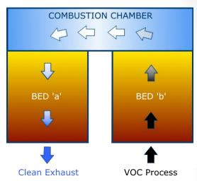
The now clean air stream next enters a second heat exchange bed where the clean stream passes directly through the media where the stream is cooled while simultaneously heating the media before being exhausted to atmosphere.
